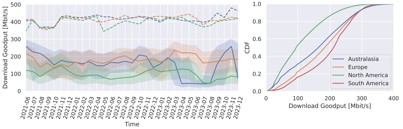
Fig. 4: Starlink goodput in the forward link (download). In the left figure, solid lines are median values; shaded areas show first and third quartiles; dashed lines are maximum values. Goodput is very variable in general. North America has lower goodputs than other countries, which is probably due to a higher subscription rate. Users from South America contributed only a few measurements (cf. Figure 3).
